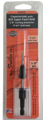
Stock # C6HTC C6 Countersink Mounted on 9/64 Taper Drill with Hex Shank See Page 11
